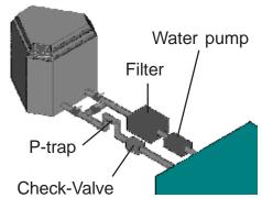
This connection method is strongly recommended to enhance the life-span of your pool heat pump.
